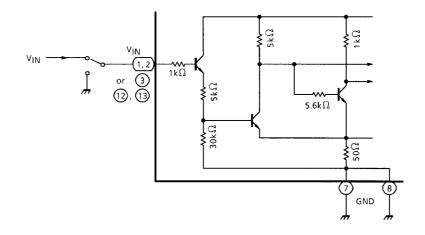
The input circuit is an active high type, as shown in the diagram. When voltage higher than the specified  $V_{IN}$  (H) is applied, the output is logic "H". When voltage lower than the specified  $V_{IN}$  (L) is applied or if the input is grounded, the output is logic "L". Since the input current IN flows to the input when logic "H", be careful with the output impedance at the previous step.
