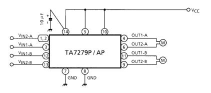
Problems may result if a capacitor is inserted in parallel to the motor.
